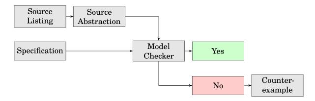
**Figure 3.1** A typical model checking pipeline. The source listing is transformed into a source abstraction suitable for verification by the model checker, along with a specification describing some property for how the software should behave. Given these two inputs, the model checker can identify a violation of the property. If a violation exists, the model checker returns a counterexample of how the property can be violated.
